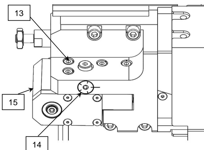
**Note 2:** A servo tuning is necessary. In the menu A2/ parameter 2021, the value (original ~7000) must be set between 2000 and 4000.
