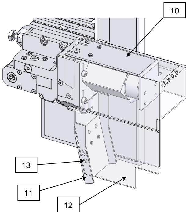
**Mark 1:** The fixing screw [13] cannot be mounted on the original sheet [11]. If needed, bore an additional passing hole in the sheet, 11.5mm below:
