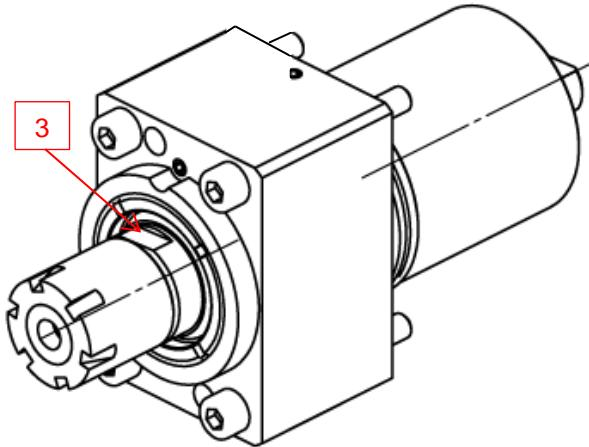
4. The tool shank diameter should never have a difference of more than 0.4 mm
