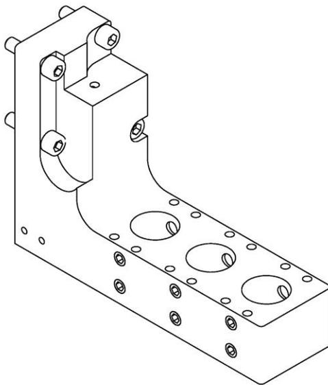
2. Then tighten lightly the fixing screws (important, make sure that the screws have the same clamping force).
