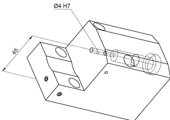
2. Then tighten lightly the fixing screws (important, make sure that the screws have the same clamping force).
